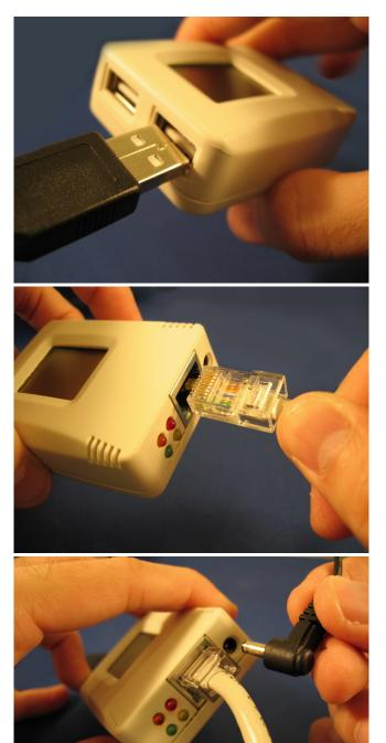
Step 2: Connect the iCAMView to LAN by using the Ethernet UTP port.
